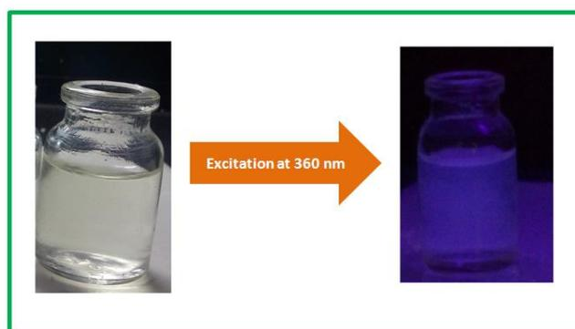
Figure 1: Photograph of zinc oxide quantum dot dispersion in ethanol
